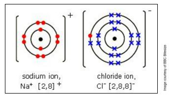
The red dot clearly shows the transferred electron from sodium to chloride to produce two ions with full outer electron shells.
