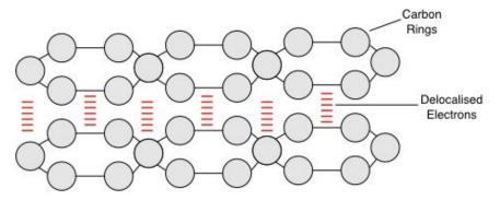
**Graphene** consists of single, **2D** sheets of graphite that are just one atom thick. These sheets are formed of hexagonal carbon rings that create a very strong, rigid material that is extremely lightweight. Delocalised electrons move through each layer allowing it to conduct electricity, making graphene a useful material in electronics.
