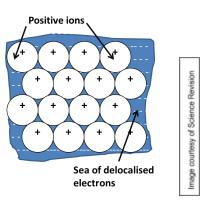
The greater the charge on the positive ion, the stronger the attractive force since more electrons are released into the 'sea'.
