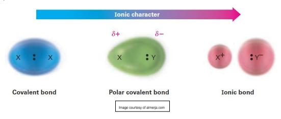
This bond polarity can be **permanent** or **induced** depending on the molecule and how it interacts with things around it.
